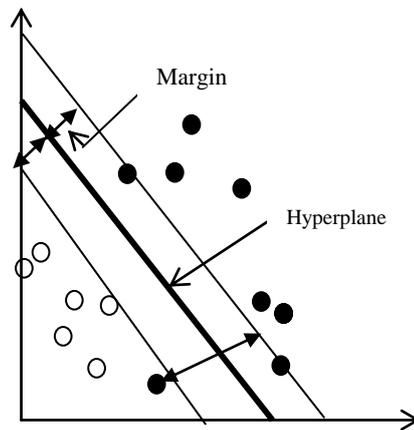
Figure 3: Support Vector Machine with a hyperplane
